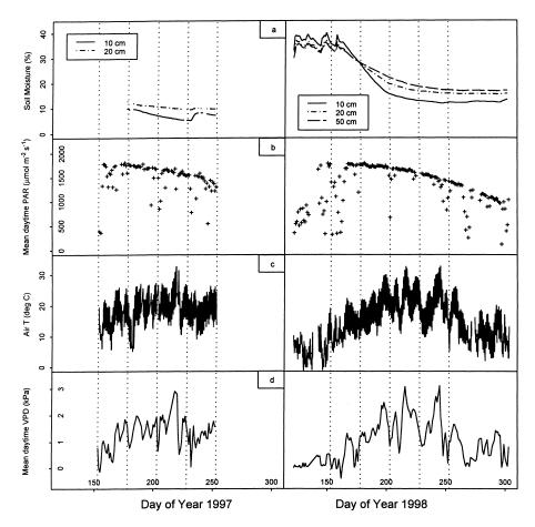
Fig. 4. Time series of environmental variables that most strongly influence  $CO_2$  and energy fluxes including (a) soil moisture, (b) daily maximum photosynthetically active radiation measured at the top of the tower, (c) air temperature measured at the top of the tower, and (d) vapor pressure deficit presented as midday (09:00–15:00 h PST) mean values. Vertical lines separate the averaging periods presented in Figs. 5 and 8.
